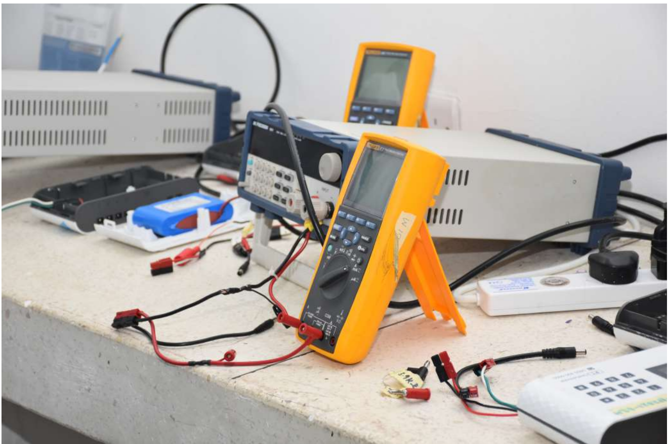
Overload protection testing setup in the solar equipment testing laboratory
